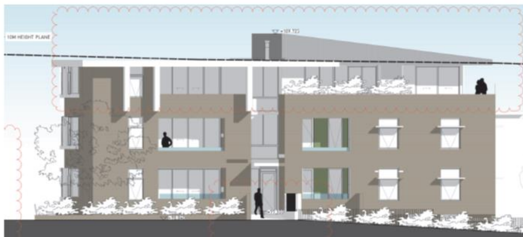
Figure 3: Amended design incorporating, lowering of finished floor levels for Building B reduces overall height.
