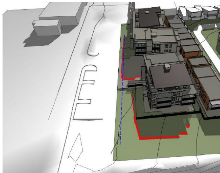
Figure 8: Shadow cast by development at 9am on 21 June, with the red showing the additional shadow cast by that part of the building above the 10m height plane.
